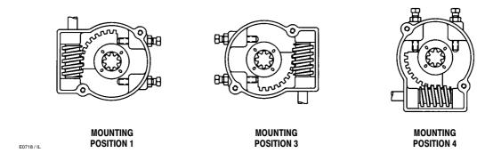
Figure 4. Direct Acting Mounting Positions (Shown in the Closed Position)
